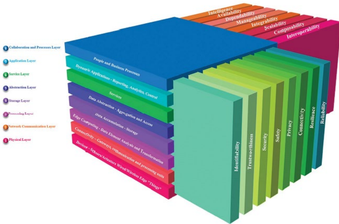
Figure 6: The general structure of CREATE-IoT 3D RAM
